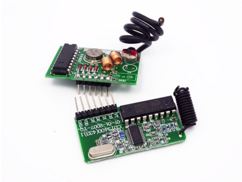
Figure 9: 433 MHz Radio Frequency Module: Transmitter and Receiver
